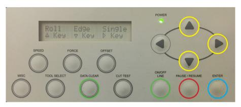
When you turn on the machine the screen will read 'Roll, Edge and Single'. You will choose for the option 'Roll' so you push the upper arrow.
