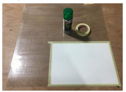
We always place the material on a trasferfoil. This ensures for good grip for the rollers whilst executing the job.
