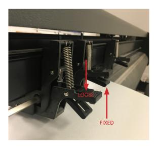
You can move the rollers by pushing down the clamps on the back of the machine and moving them to the left of right. Pulling them back up fixes the position of the rollers.
