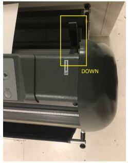
At the right side of the machine you find a lever. Putting it in the upright position will levetate the rollers which makes it possible to place the transferfoil with your material. After you placed your material you lower this lever, clamping your material between the rollers.
