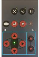
If the orange LED near the on/off button is turned on, the machine is turned off.
