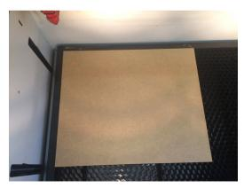
Position your material always in the top left corner on the honeycomb table. The table is constructed in a way that it clicks into two fixed rulers in the lasercutter. Always verify that the honeycomb table is positioned correctly.
