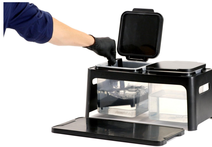
Clean parts in isopropyl alcohol (IPA) to remove any uncured resin.
