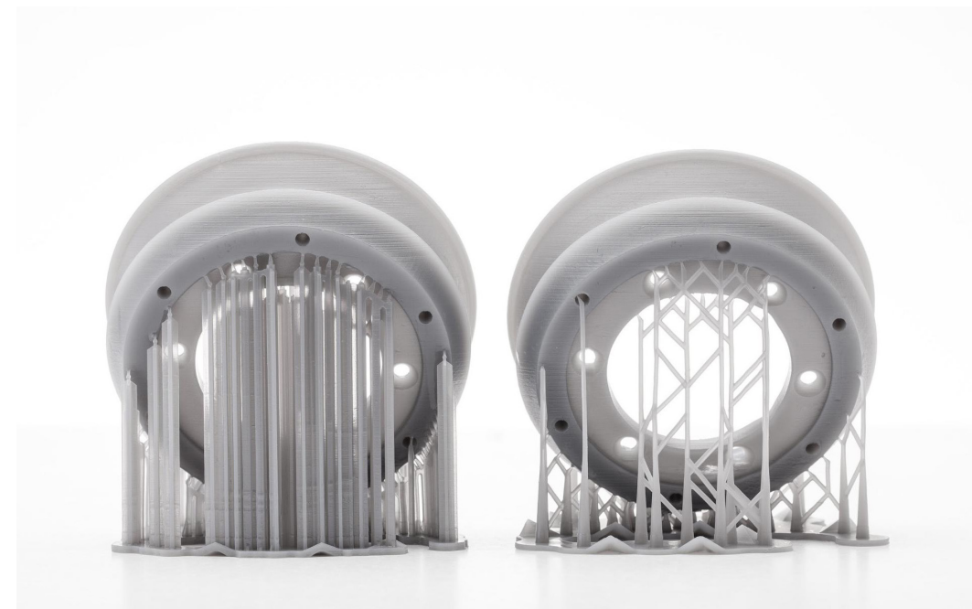
Both SLA systems use support structures to attach parts to the build platform.
