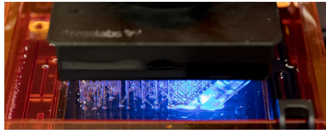
Stereolithography printing in progress.
